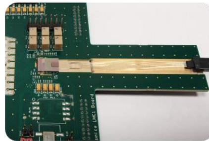
*24-channel polymer packaging substrate coupled to a Si photonic chip*
