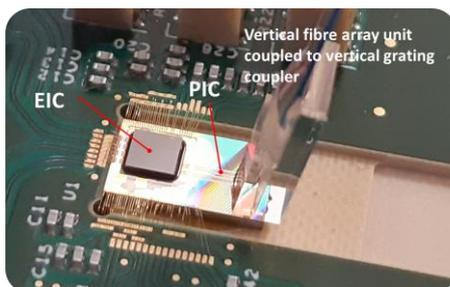
*100 Gb/s per fiber 2-channel CWDM transceiver*
